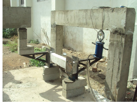
Fig: Typical setup For Shear & Torsion Test.
